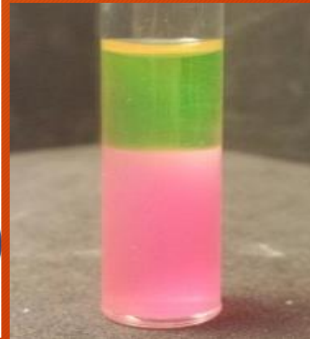
a Segregative phase separation results in: Two immiscible liquid phases
